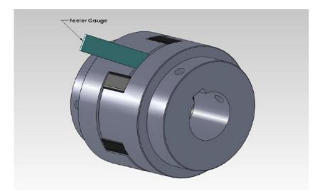
It is very important to maintain a gap of 0.070" to 0.10" between the two halves of the coupling to achieve proper pump operations and avoid any pump failures. Please use a feeler gauge as shown in the picture to maintain this gap.
