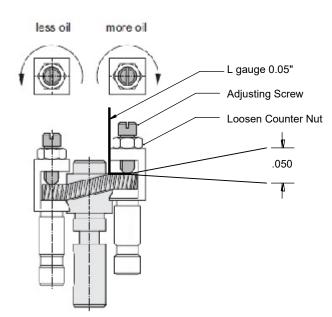
RCF500 oil pumps come pre adjusted from the factory and rarely require any adjustment during their life time. However if a need arise, the following procedure should be followed to adjust the oil flow rate.
